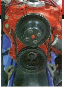
We ran the engine on the dyno with the OEM-style mechanical water pump driven by a pulley set at about a 1:1 ratio to crank rom.
