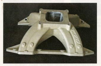
The manifold complements the cylinder heads, and here we opted for the top end charge of a single-plane Edelbrock Victor. For more low and mid range power, the RPM intake would be a better choice.
