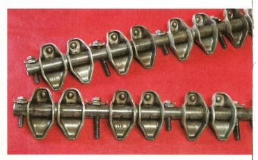
The factory stamped steel rocker setup looks primitive, but it is very lightweight and effective. We simply cleaned off the stockers for reuse in our 440.
