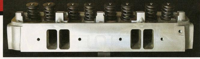
The cylinder heads are a key part to power production. For an application like this it is hard to beat the Edelbrock RPM heads. These heads feature far improved flow in comparison to the OEM heads, and we find the quality control very good right out of the box.
