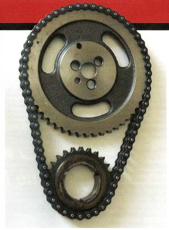
To drive the cam we used a COMP roller timing set. This standard set comes with three keyways at the crank gear to adjust the cam timing +/-4 degrees. Further fine-tuning of the cam timing will require the use of offset bushings at the cam gear indexing pin.
