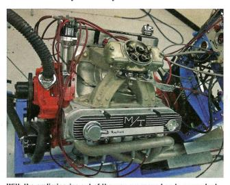
With the preliminaries out of the way, we moved on to power testing. The engine pulled strongly to above 6,000 rpm, and delivered very impressive torque throughout the test range. Power was substantial, showing 537 hp at 5,800 rpm
