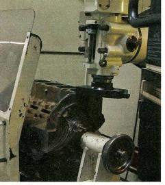
We kept the block machining to only the necessary operations. A bore, hone, and deck job sums up the major block machining.
