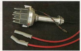
For dyno testing purposes, our favored distributor setup is the MSD Pro Billet. Although not a bargain piece, it is incredibly reliable, and plugs right into the dyno installation. For street use, a Mopar Performance vacuum advance distributor is a viable alternative.
