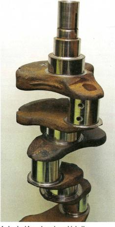
A standard forged crank went into the bottom end for our build. The crank simply received a .010-inch grind on the journals, and was installed with a set of Clevite bearings.
