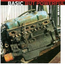
When it comes to 440 Mopar engines, any usable core is a suitable starting point for a high-performance build, but the earlier engines have the advantage of a very good forged steel crankshaft.
