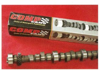
A flat tappet hydraulic cam is far and away the most cost-effective setup in a mild performance engine, especially if the OEM valve-train is retained. This COMP XE285HL is a fairly radical stick.
