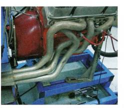
Exhaust is another important factor in making good output. These 1<sup>7</sup>/<sub>8</sub>-inch Hooker Comp headers are sized about perfectly for a 440 in the 450-550 hp range.
