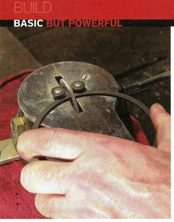
Experience has shown that moly faced rings provide much improved bore life compared to the cheap "rebuilders" iron ring. These Speed-Pro rings are also much more durable than plain cast-iron rings and provide a power advantage.
