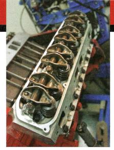
After the initial break-in and calibration runs, we took the time to change the oil to a fresh fill, and go through an inspection process before proceeding with the power tests. The valve covers were pulled and the stock rockers were holding up fine.
