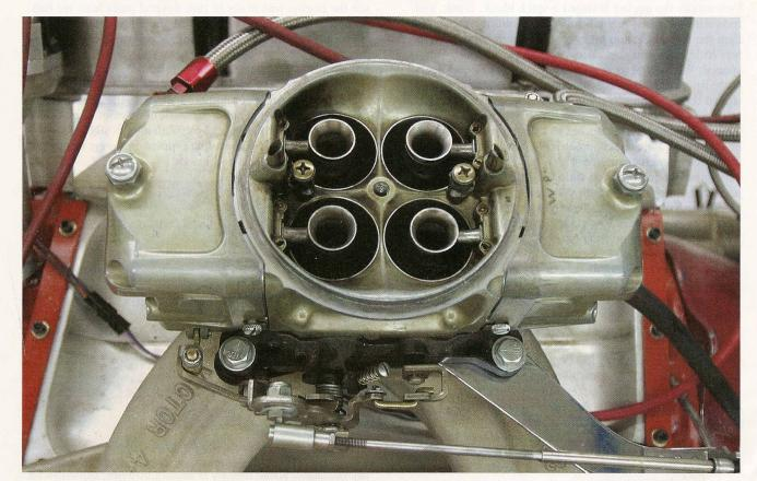
For carburetion on the dyno, we went with the largest 4150-style carb on hand, the Race Demon RS with the large 975-cfm sleeves installed. This carb would perhaps be overkill on the street, but a more moderate carb can be substituted with a minimal impact on power.
