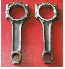
Mopar OEM 440 rods came in two basic configurations, the much more common standard rod, marked "LY" on the beam (right), and the heavy duty rods used after 1970 on HP engines (left). Either can handle the power of a hot street combination with resizing and fresh high-strength bolts.
